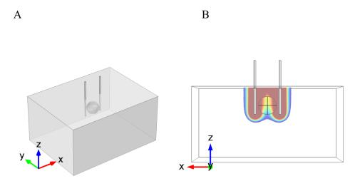
**Figure 1:** (A) Simple 3D model of tumor and needle electrodes in healthy tissue; (B) electric field over reversible threshold inside the healthy tissue and the tumor.
